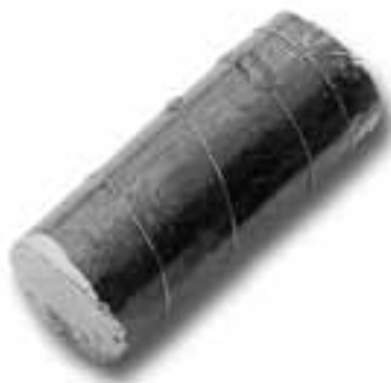
Hipped sample of TIMREX® Graphite (HIP, 350 Mpa, 1900°C) with thermocouples
