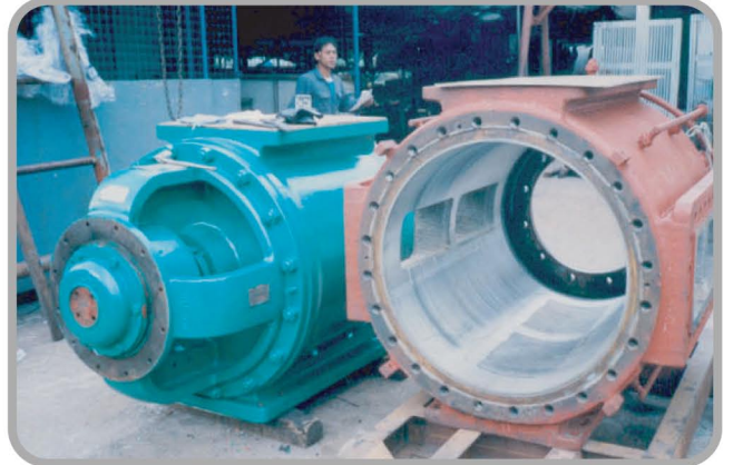
LOW PRESORE FEEDER & HIGH PRSSURE FEEDER
